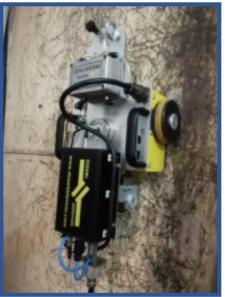
• Reliable automated inspection of storage tank walls for corrosion degradation
