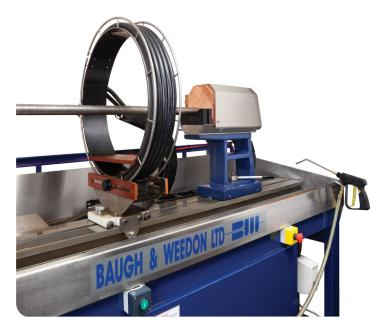
bench. Output sockets allow the bench power supply to be connected to prods, leeches or wrapped cables.
