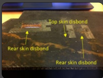
Figure 3: Thin CFRP honeycomb sample with rear surface disbonds.
