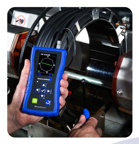
**Shot Timer Mode:** Tracks magnetising shot duration and records max Gauss levels for precise MPI testing.
