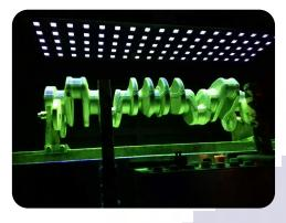
**Apollo 365L** overhead panel utilizes the state-of-art LED technology and makes it a great tool for fluorescent MT, PT and leak detection. The unique feature of Apollo 365 series LED UV panel is its module-based design. Each LED of Apollo 365 is encapsulated as an independent unit and are interchangeable, between "flood" and "spot" for example, so you can create your preferred overhead light configuration with the desired UV intensity and coverage area.
