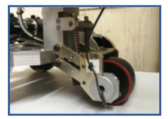
data The acquisition system measures the thicknesses every 1 with accurate control mm position and measurement accuracy better than 0.1 mm. The real time display shows the Adata with either the thickness or amplitude scans in the B-Scan window (switchable). All A-scans are stored for future analysis and a B Scan thickness and amplitude presentations can be provided from the A scan data.
