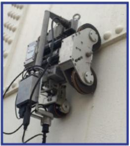
Reliable automated inspection of storage tank walls for corrosion degradation
