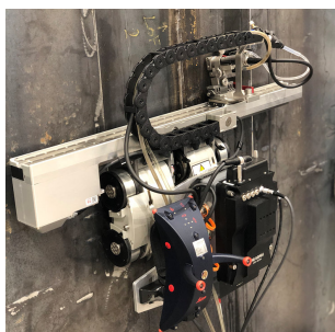
Light enough to be mounted on a magnetic-wheel scanner, to simplify the umbilical. Shown here on a Jireh scanner, alongside a Hexagon Leica T-Probe laser target.
