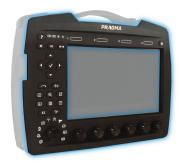
The UNITOP silicone keypad provides a nice tactile feedback and will prevent dirt adherence. The keypad maintains its feel and performance over a wide temperature range. The protective glass is scratchproof.
