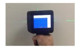
The live display allows real time alignment, observation and measurement of surface and sub-surface features.
